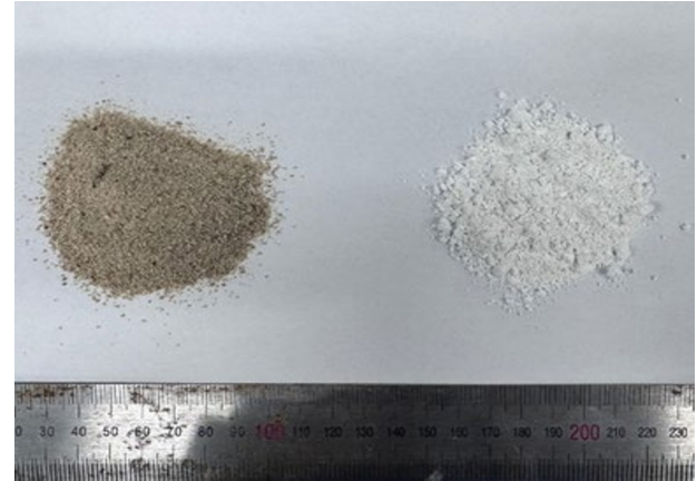
Fig. 1. Na-Bentonite (expansive clay)–(left) and Kaolinite (non-expansive clay)–(right).
