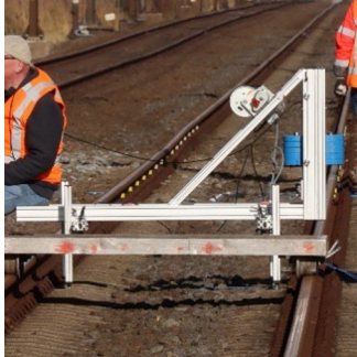
Fig. 1. Overview of the falling weight impact test equipment on the railway track.
