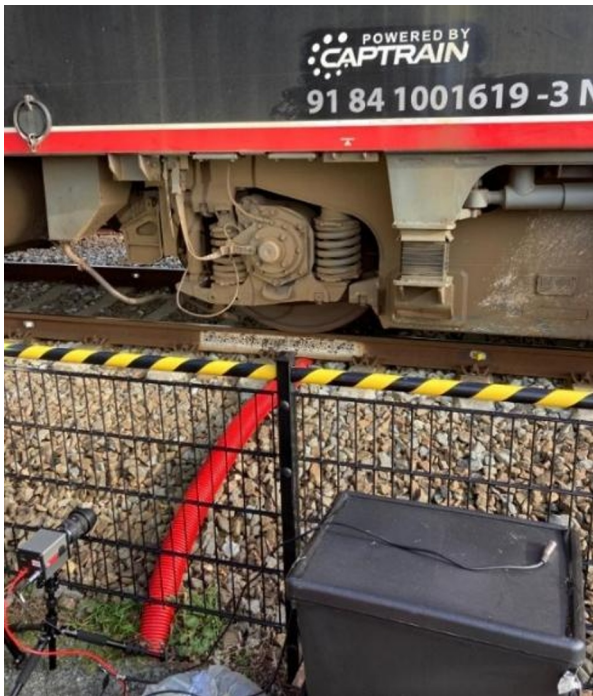
Fig. 5. Test train wheel at measurement location, camera on left hand side measuring speckle pattern on outer rail at test location Delft Schiedam.
