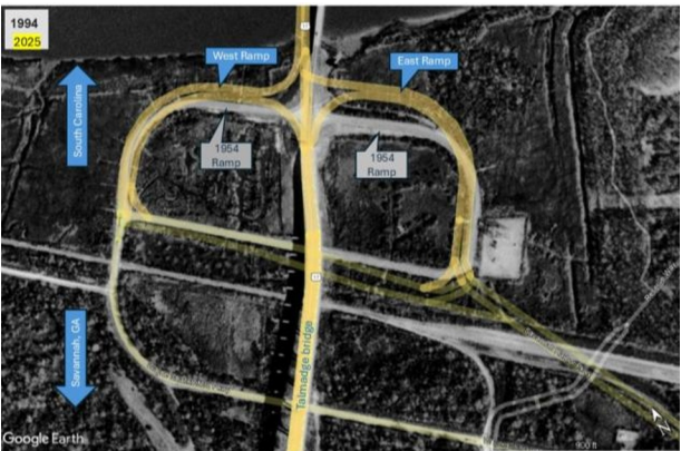
Fig. 2. Ramp layout relative to 1954 ramps.
