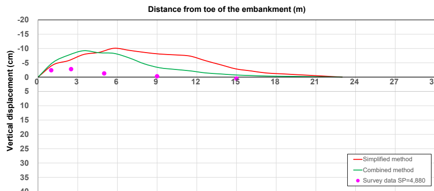
Fig. 8. Comparison of the influence degree of surrounding ground on embankments using the simplified method and the combined method.
