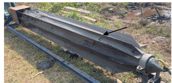
Fig. 11. Soil adhered at the base surface after retrieval from the ground. Test carried out after 43 h installation.
