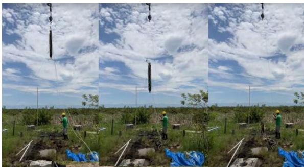
Fig. 8. BT-1000 Model (1/10 scale) launching in Sarapuí II test site.
