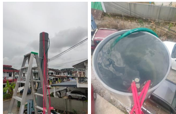
Fig. 4. Piezometer calibrated in the PVC column.
