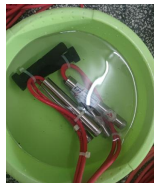
Fig. 5. Piezometer was saturated before installation.
